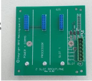
This connector enables remote expansion modules to be connected to the PLC mainframe. This backplane is supplied with the mating connector (not shown in the photo).
