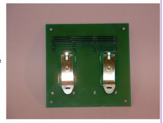
Engage the top hooks of the clips over the top lip of the rail.
