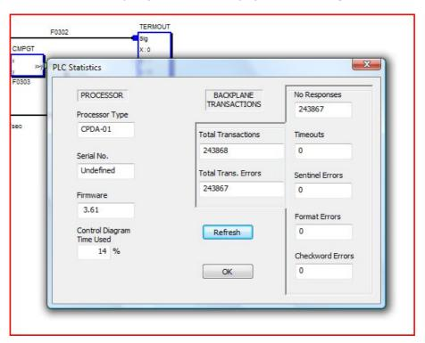
In the case above, the serial number had not been embedded into the CPDA-01. Production units have the serial number embedded as part of the test and calibration process. The system being examined here carried a control diagram which called for input from an EXDA-01 Expansion Module in Slot 1. However no module was fitted, so the No-Response count is almost 100%.
