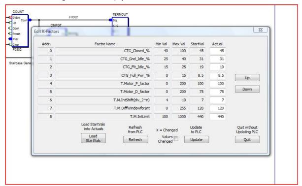
The 'Up' and 'Down' buttons allow you to scroll through a file which contains more than 9 items. You can have up to 128 K-Factors in any project.
